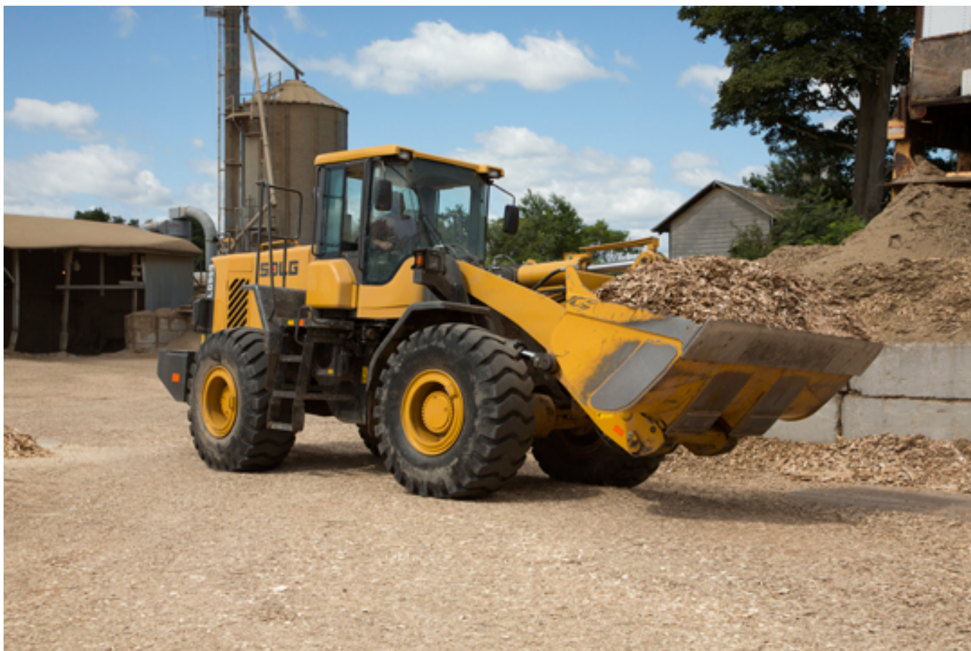
The LG959 flexes its 4.0 yd 3 bucket, hauling a large load of wood tips across the production yard.
